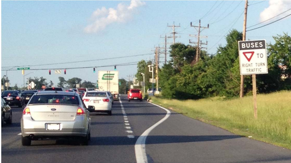
Figure 43. Photo. Maryland SHA sign to manage right-turn lane conflict. (Source: Kittelson and Associates, Inc.)
